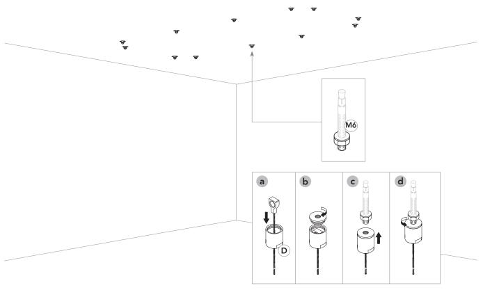
4 Determine the correct height of the OneFrame frame to grid clip, depending on the tile edge.
