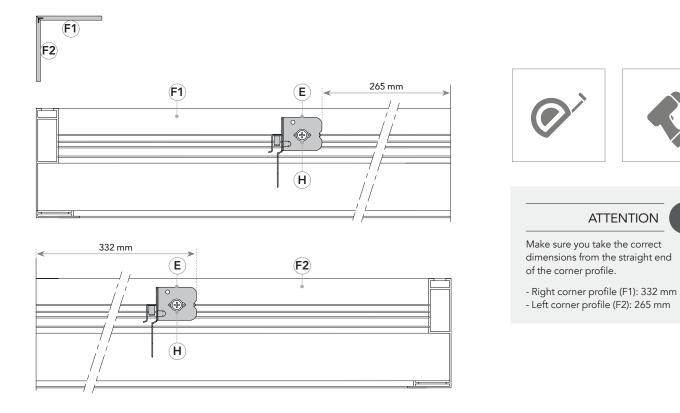
6 Connect and close the OneFrame extension and corner profiles with the length connectors, corner pieces and TEK screws.
