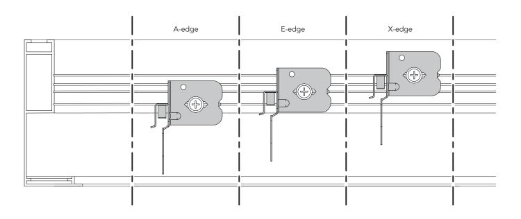
5 Install the OneFrame frame to grid clips on the OneFrame corner kit.
