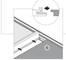
Place tile (c) and slide the tile against the Z-profile. This Z-profile doesn't need to be fixed with angle brackets.
