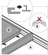
Install the Z-profile and slide the Z-profile in the groove of the tile. This Z-profile doesn't need to be fixed with angle brackets.
