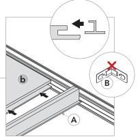
Slide the second Z-profile in the groove of the second tile (b).
