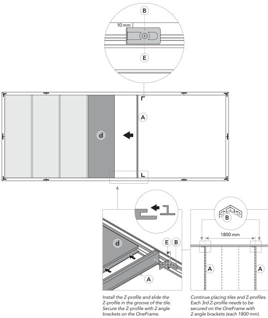
Continue placing tiles and Z-profiles. Each 3rd Z-profile needs to be secured on the OneFrame with 2 angle brackets (each 1800 mm).
