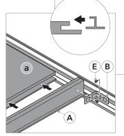
Install Tile (a) and slide the Z-profile in the groove of the tile. Secure the Z-profile with 2 angle brackets on the OneFrame.
