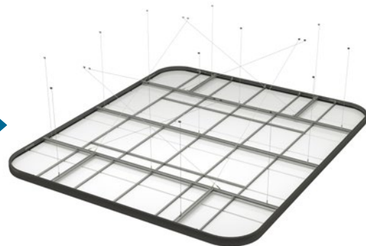
6. Install X-edge tiles.
